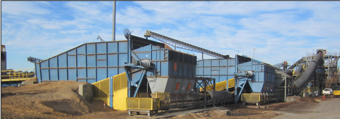
Figure 4-6 Rear View of Back-on Style Truck Tipper with Near Grade Dumper Hopper (Drax Morehouse Facility)
