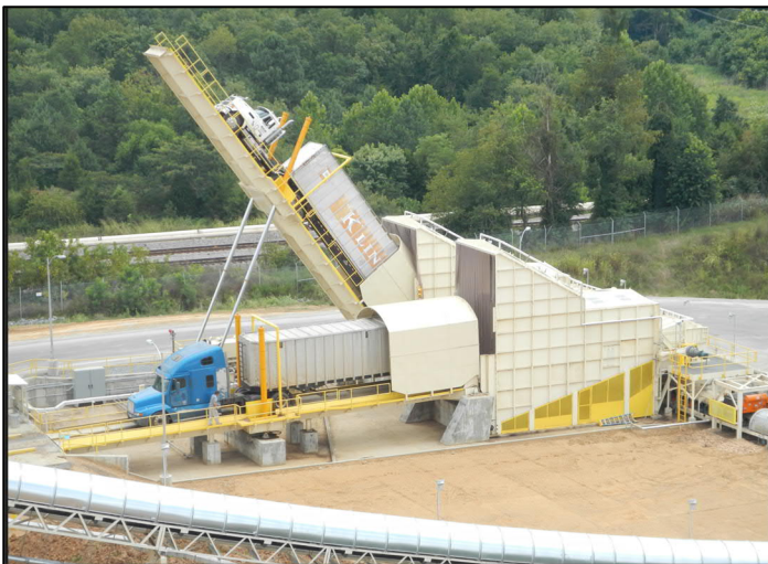
Figure 4-1 Back-on Style Truck Tipper with Dumper Hopper and Dust Collection (courtesy of Bruks)
