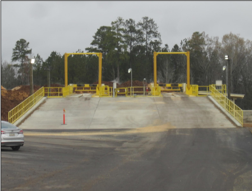
Figure 4-2 Back-on Style Truck Tipper with no Dumper Hopper or Dust Collection (Demopolis)
